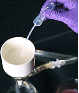
• Prepare to filter your sample by placing a filter paper in the Buchner funnel and wetting it with clean solvent.
