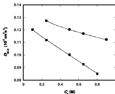
Fig. 2. Lysozyme diffusion coefficient,  $D_{DLS}$ , as a function of salt concentration ( $\bullet$ , NaCl;  $\blacksquare$ ,  $\text{Na}_2\text{SO}_4$ ) at 25 °C, pH 4.5 and constant protein concentration: 0.6 mM. The solid curves are smoothed curves through the points.
