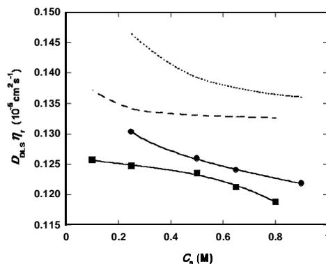
Fig. 3. Viscosity-corrected diffusion coefficients,  $\eta_r D_{DLS}$ , as a function of salt concentration ( $\bullet$ , NaCl;  $\blacksquare$ ,  $\text{Na}_2\text{SO}_4$ ). The solid curves are smoothed curves through the points. The dashed curves ( $\cdots$ , NaCl;  $--$ ,  $\text{Na}_2\text{SO}_4$ ) are the Nernst-Hartley predictions.
