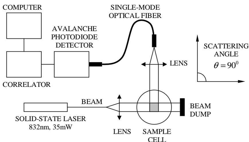
Fig. 1. Scheme of the DLS apparatus used for measurements of lysozyme diffusion coefficients.
